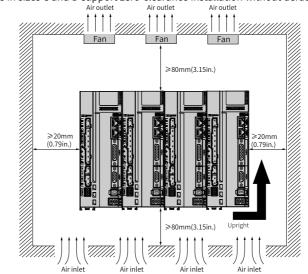
Servo drives in sizes C and D support zero-clearance installation without derating.
