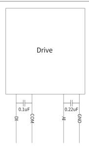
Figure 7-2 I/O signal cables with capacitance increased
