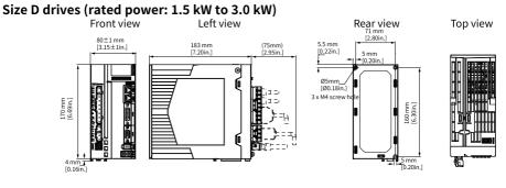
Figure 3-8 Dimensions of Size D
