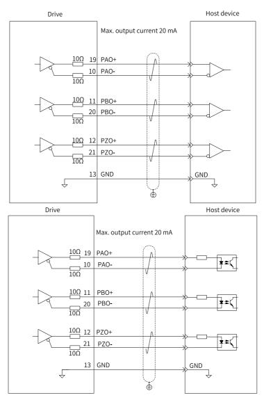
Encoder phase Z output circuit outputs OC signals. Typically, this circuit provides feedback signals to the host controller in a position control system. An optocoupler circuit, relay circuit, or bus receiver circuit shall be used in the host controller to receive feedback signals.
