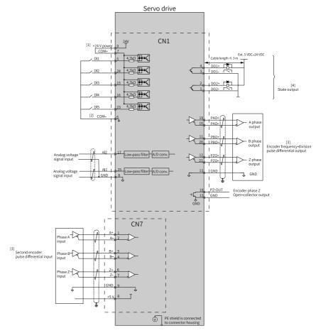
Figure 5-1 Electrical Wiring Diagram
