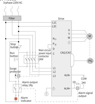
Figure 6-4 Main circuit wiring
