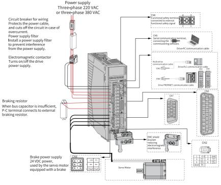
Figure 4-1 System wiring example
