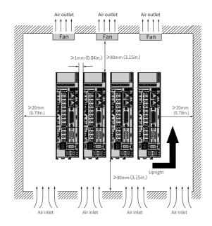
Figure 3-4 Clearance for compact installation
