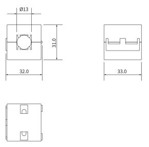
Figure 2-7 Dimensions of the ferrite clamp
