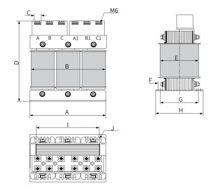
Figure 2-3 Dimensions of 40 A (1.45 mH) AC input reactors Table 2–5 Dimensions of Inovance AC input reactors (unit: mm)
