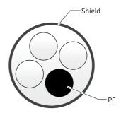
Figure 6-7 Four-core shielded cable
