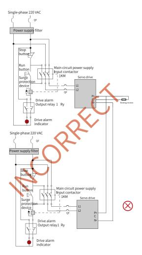
Figure 4-6 Wrong common DC bus connection of two drives with different AC input
