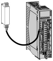
Figure 3-12 Connection of the EMC filter
