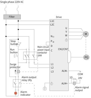
Figure 6-3 Main circuit wiring of single-phase 200 V models
