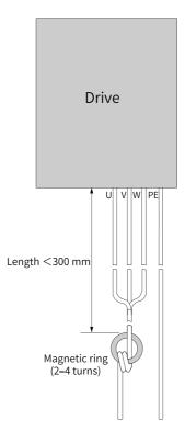
Figure 3-13 Installing the magnetic ring
