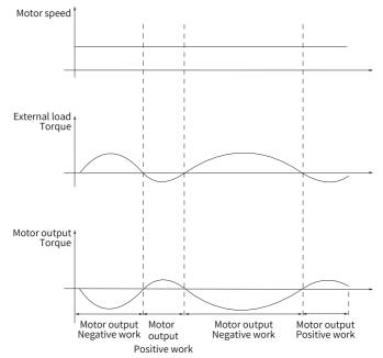
Figure 2-10 Example of the curve with external load torque
