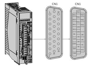
Figure 6-8 Control terminal pin layout (CN1)
