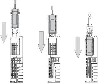
Figure 3-16 Installing the battery box (bottom view)
