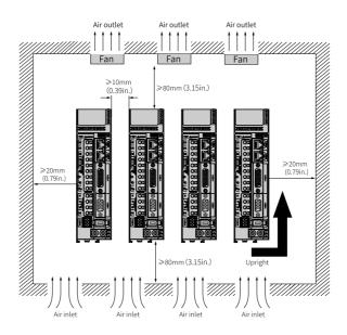
Figure 3-3 Clearance for side-by-side installation
