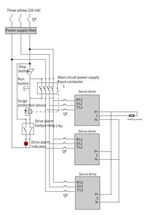
Figure 4-3 Topology of three-phase 220 VAC/380 VAC input common DC bus
