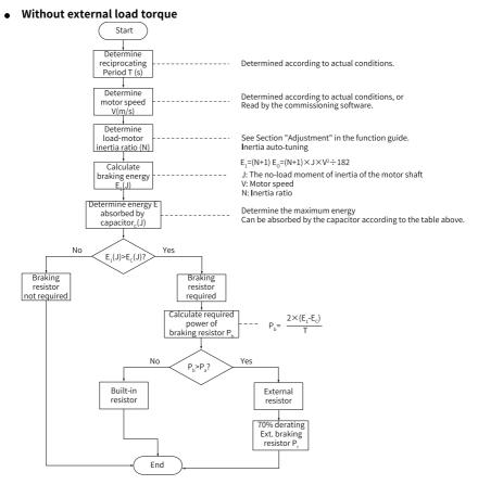
Figure 2-9 Flowchart for selecting the braking resistor
