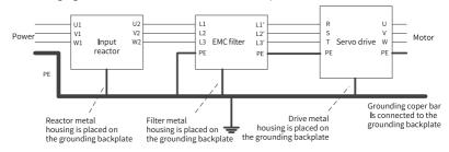
The following figure shows the connection of the AC input reactor.
