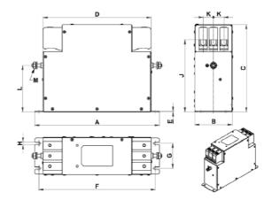
Figure 2-5 Dimension drawing of FN 3287 series filters (unit: mm) Table 2–9 Dimensions of FN 3287 series filters (unit: mm)
