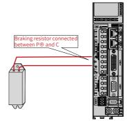
Figure 6-19 Wiring of external braking resistor
