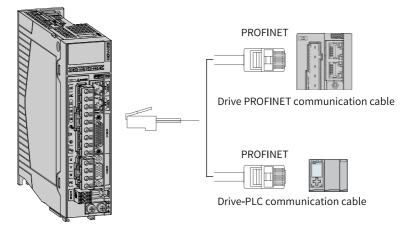
Figure 6-15 Wiring of communication cables
