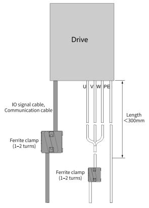
Figure 3-14 Installation of the ferrite clamp
