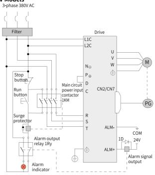
Figure 6-5 Main circuit wiring
