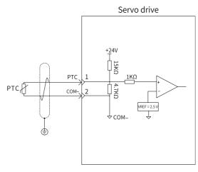
Figure 6-17 PTC wiring diagram
