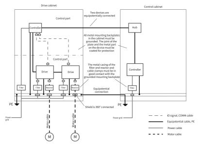
Figure 6-6 Recommended wiring for the control cabinet system
