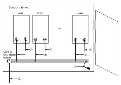
Table 6–3 Description for grounding of multiple drives installed in parallel
