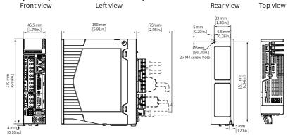
Figure 3-6 Dimensions of Size A
