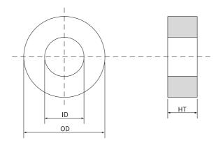
Figure 2-6 Dimensions of the magnetic ring
