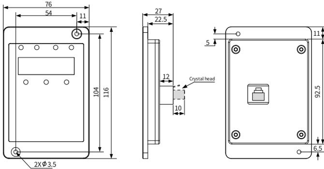
Figure 2-2 Mounting dimensions of MD32NKE1 (unit: mm)
