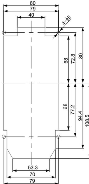
Figure 2-5 Sheet metal slot dimensions (unit: mm)
