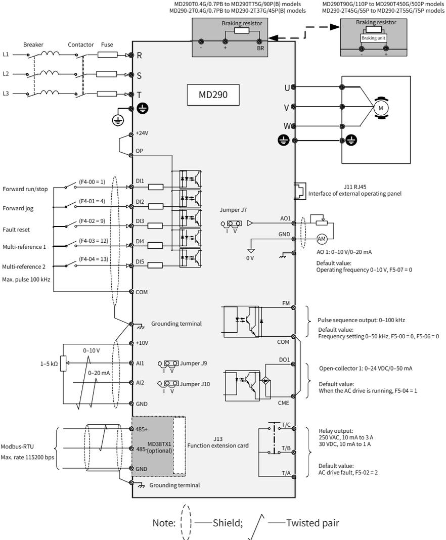
Figure 3-8 Typical wiring
