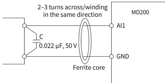
Figure 2-5 Installing a ferrite core
