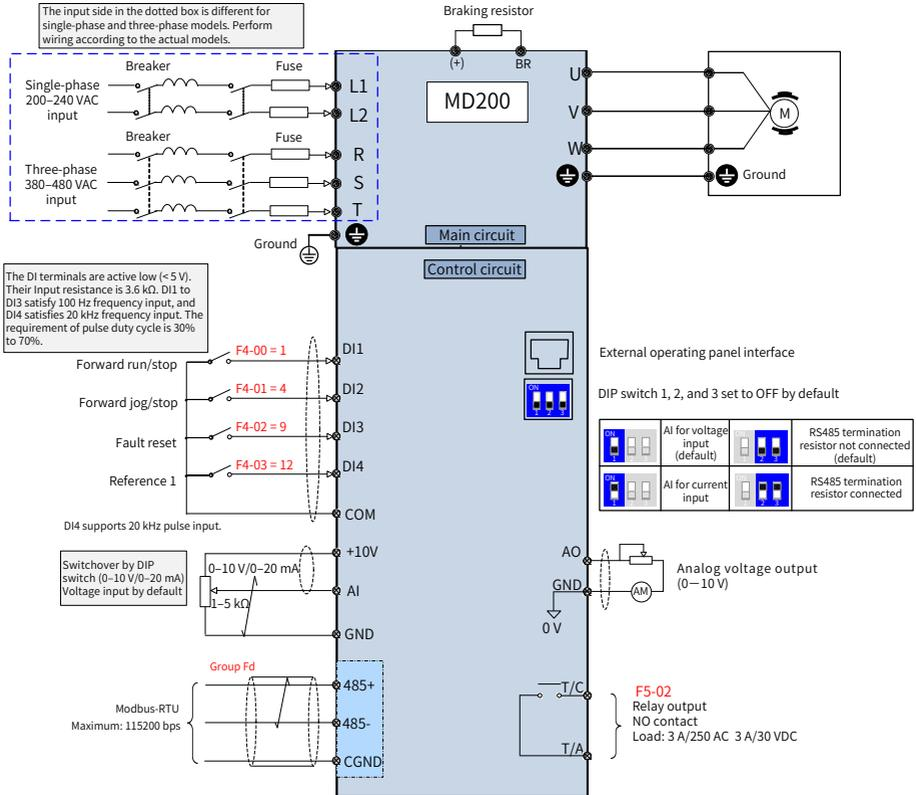
Figure 2-2 Wiring diagram of the single-phase/three-phase (MD200S0.4B to MD200S2.2B and MD200T0.4B to MD200T3.7B) power input terminals
