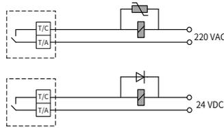
Figure 2-10 Anti-interference processing of relay output terminals
