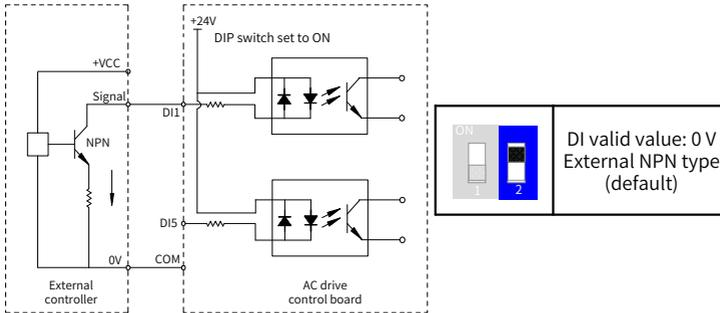
Figure 2-6 Sink wiring
