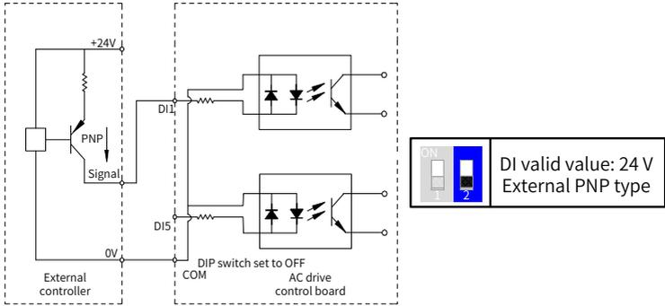
Figure 2-8 Source wiring
