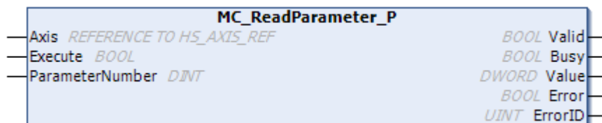
Figure 6-25 Diagram of the MC_ReadParameter_P function block
