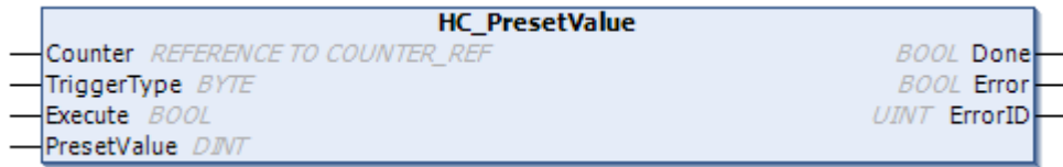
Figure 6-3 Diagram of the HC_PresetValue function block
