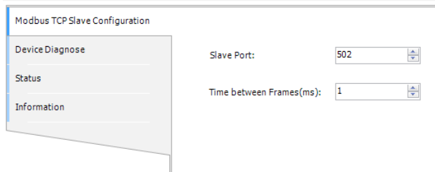
Figure 3-49 Modbus TCP slave configuration
