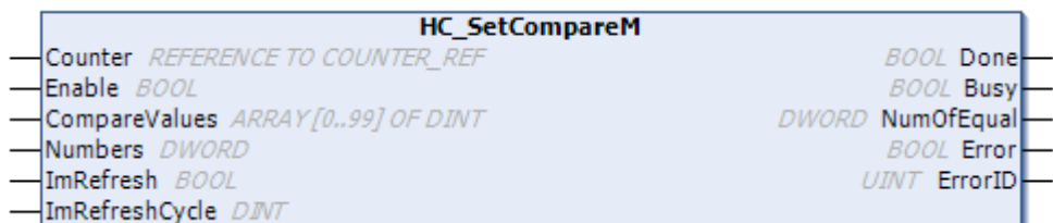
Figure 6-12 Diagram of the HC_SetCompareM function block
