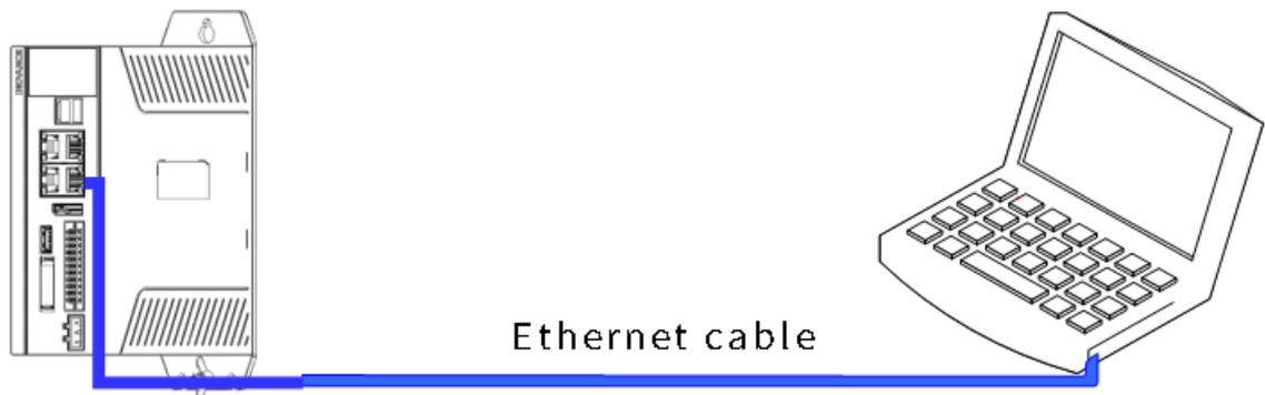
The controller can also be connected to a hub or switch through the Ethernet cable, enabling multi-point connection with other network devices.
