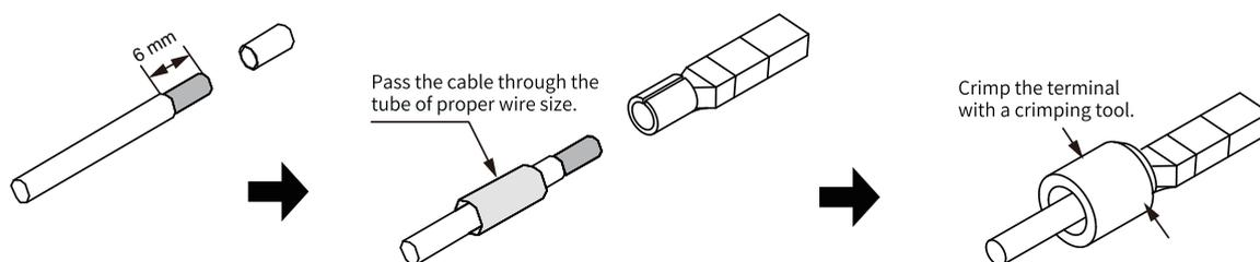
For the 2\*6-pin dual-row connector used for I/O and communication, the requirements are as follows:
