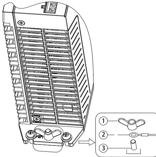
① - Wing nut; ② - Grounding cable; ③ - Grounding screw
